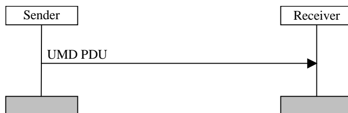
Figure 11.2: Unacknowledged mode data transfer procedure
