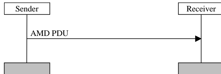
Figure 11.3: Acknowledged mode data transfer procedure
