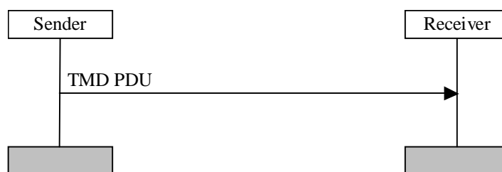
Figure 11.1: Transparent mode data transfer procedure
