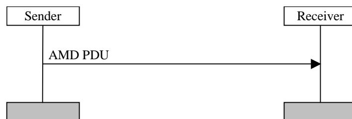
Figure 11.3: Acknowledged mode data transfer procedure
