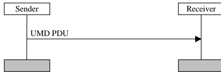
Figure 11.2: Unacknowledged mode data transfer procedure
