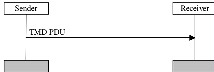
Figure 11.1: Transparent mode data transfer procedure
