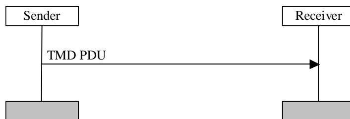
Figure 11.1: Transparent mode data transfer procedure
