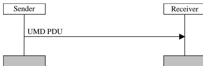
Figure 11.2: Unacknowledged mode data transfer procedure
