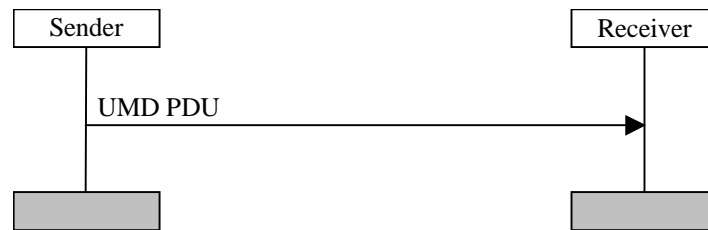
Figure 11.2: Unacknowledged mode data transfer procedure
