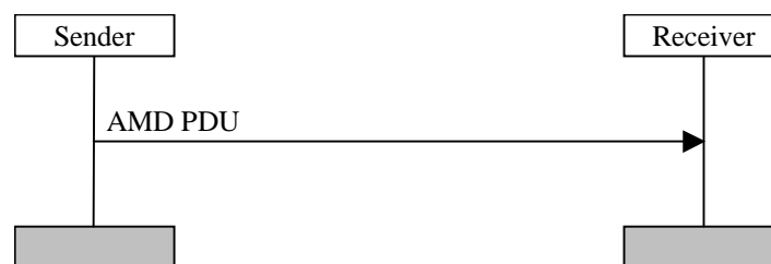
Figure 11.3: Acknowledged mode data transfer procedure
