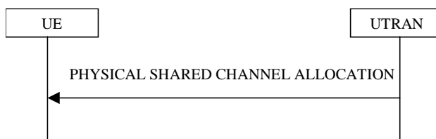
Figure 8.2.7-1: Physical Shared Channel Allocation
