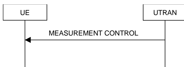
Figure 8.4.1-1: Measurement Control, normal case
