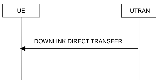
Figure 8.1.9-1: Downlink Direct transfer, normal flow
