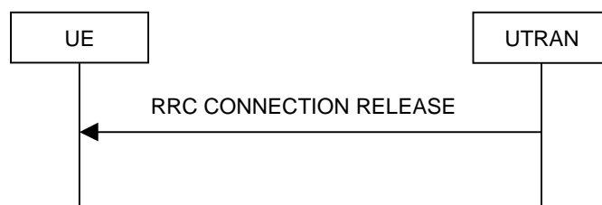
Figure 8.1.4-2: RRC Connection Release procedure on the CCCH
