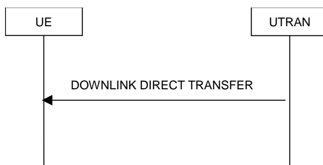
Figure 8.1.9-1: Downlink Direct transfer, normal flow
