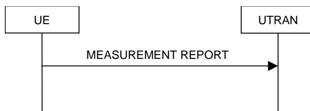
Figure 8.4.2-1: Measurement report, normal case
