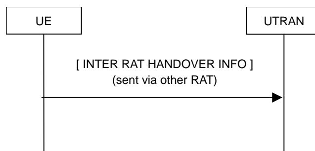
Figure 8.1.16-1: Inter RAT handover information transfer, normal flow
