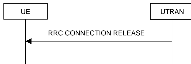
Figure 8.1.4-2: RRC Connection Release procedure on the CCCH
