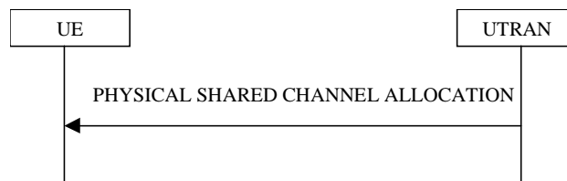
Figure 8.2.7-1: Physical Shared Channel Allocation
