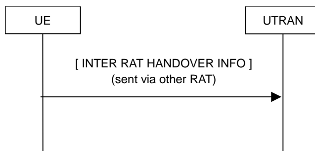
Figure 8.1.16-1: Inter RAT handover information transfer, normal flow
