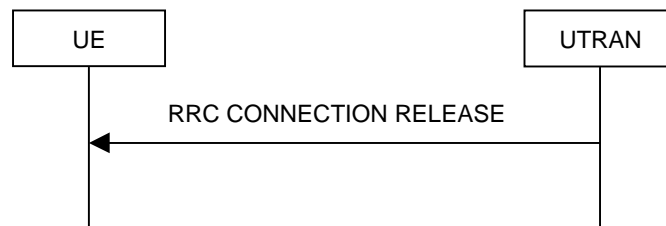
Figure 8.1.4-2: RRC Connection Release procedure on the CCCH
