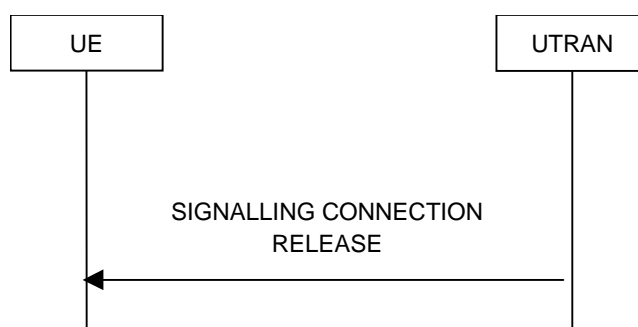
Figure 8.1.13-1: Signalling connection release procedure, normal case
