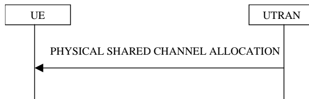
Figure 8.2.7-1: Physical Shared Channel Allocation
