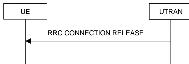
Figure 8.1.4-2: RRC Connection Release procedure on the CCCH
