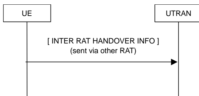
Figure 8.1.16-1: Inter RAT handover information transfer, normal flow
