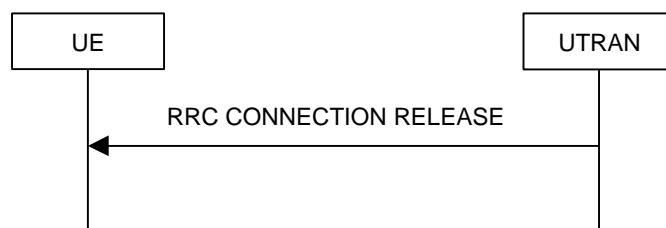
Figure 8.1.4-2: RRC Connection Release procedure on the CCCH
