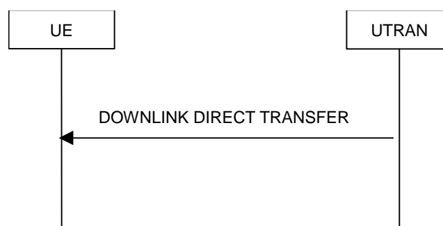
Figure 8.1.9-1: Downlink Direct transfer, normal flow
