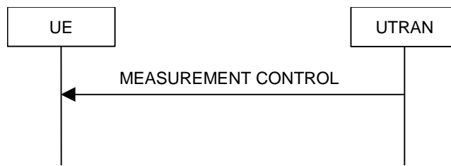
Figure 8.4.1-1: Measurement Control, normal case
