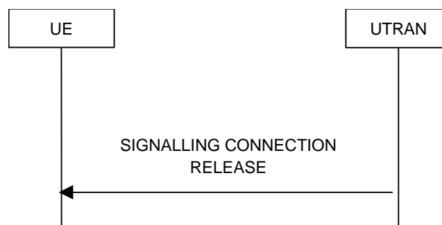
Figure 8.1.13-1: Signalling connection release procedure, normal case
