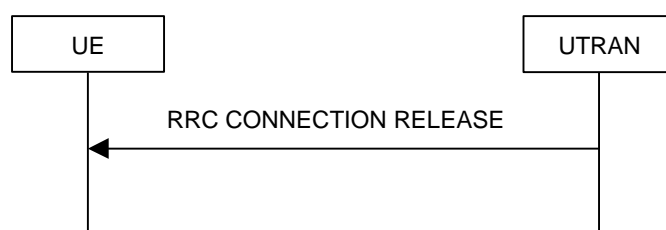
Figure 8.1.4-2: RRC Connection Release procedure on the CCCH
