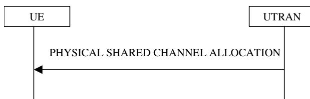
Figure 8.2.7-1: Physical Shared Channel Allocation
