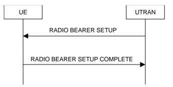
Figure 8.2.2-1: Radio Bearer Establishment, normal case
