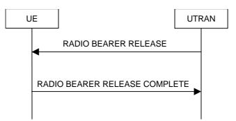
Figure 8.2.2-5: Radio Bearer Release, normal case
