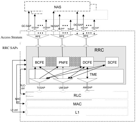
Figure 4.2-1: UE side model of RRC
