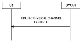
Figure 8.2.10-1: Uplink Physical Channel Control
