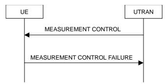
Figure 8.4.1-2: Measurement Control, failure case
