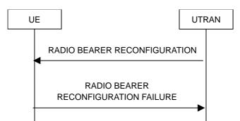
Figure 8.2.2-4: Radio bearer reconfiguration, failure case
