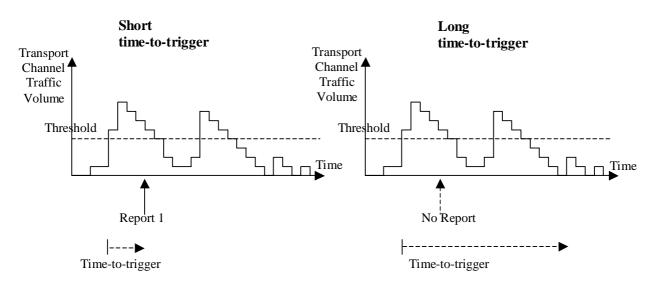
Figure 14.4.3.1-2: Time-to-trigger is used to achieve time hysteresis
