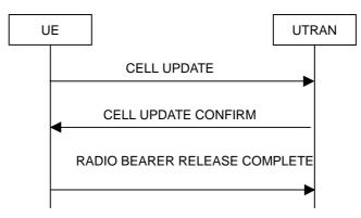
Figure 8.3.1-5: Cell update procedure with radio bearer release
