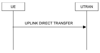
Figure 8.1.10-1: Uplink Direct transfer, normal flow
