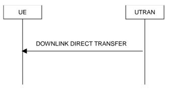
Figure 8.1.9-1: Downlink Direct transfer, normal flow
