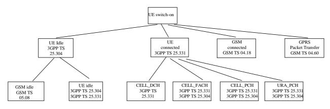
Figure 4.1-1: Mapping of UE state to 3GPP Specifications
