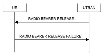
Figure 8.2.2-6: Radio Bearer Release, failure case
