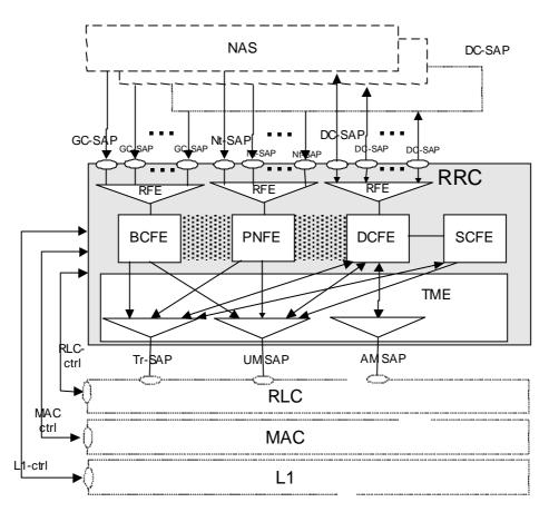
Figure 4.2-3: UTRAN side RRC model (DS-41 System)
