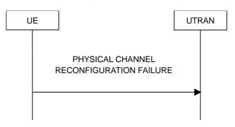
Figure 8.2.11-1: Physical channel reconfiguration failure in case of runtime configuration error
