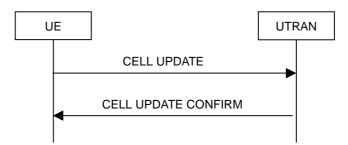
Figure 8.3.1-1: Cell update procedure, basic flow
