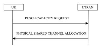
Figure 8.2.8-1: PUSCH Capacity request procedure
