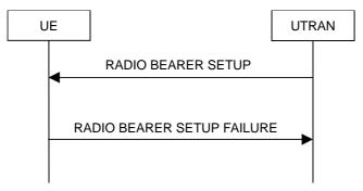
Figure 8.2.2-2: Radio Bearer Establishment, failure case
