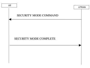
Figure 8.1.12-1: Security mode control procedure
