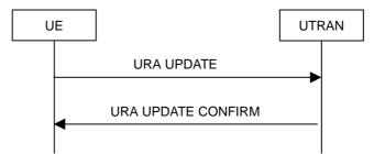
Figure 8.3.1-8: URA update procedure, basic flow
