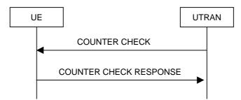
Figure 8.1.15-1: Counter check procedure
