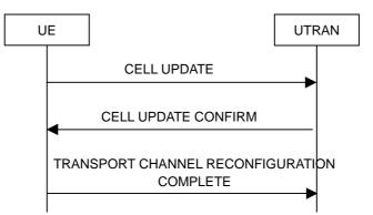
Figure 8.3.1-4: Cell update procedure with transport channel reconfiguration
