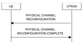
Figure 8.2.2-9: Physical channel reconfiguration, normal flow
