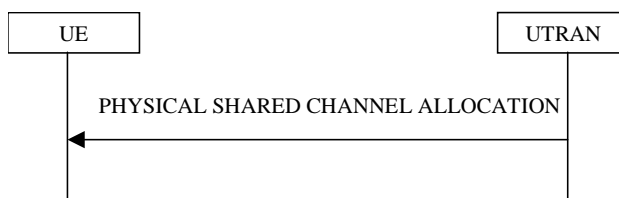
Figure 8.2.7-1: Physical Shared Channel Allocation
