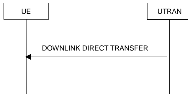
Figure 15: Downlink Direct transfer, normal flow
