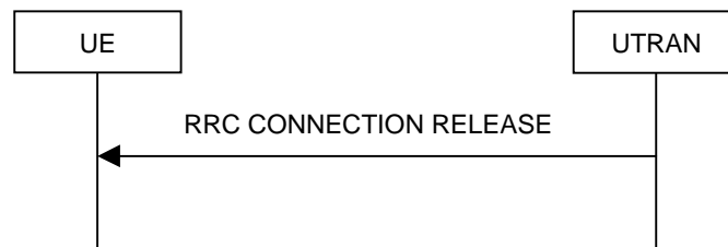
Figure 11: RRC Connection Release procedure on the CCCH
