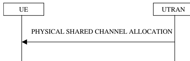
Figure 34: Physical Shared Channel Allocation
