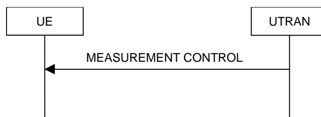
Figure 56: Measurement Control, normal case
