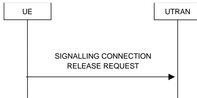
Figure 20: Signalling connection release request procedure, normal case
