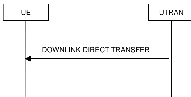
Figure 15: Downlink Direct transfer, normal flow
