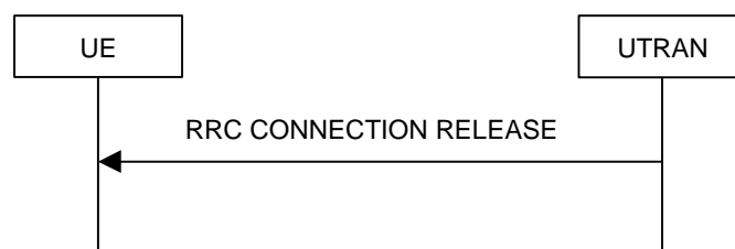
Figure 11: RRC Connection Release procedure on the CCCH
