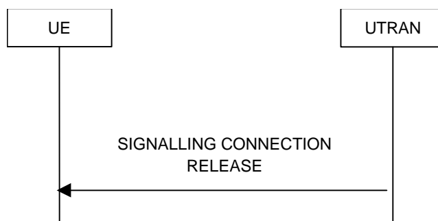
Figure 19: Signalling connection release procedure, normal case
