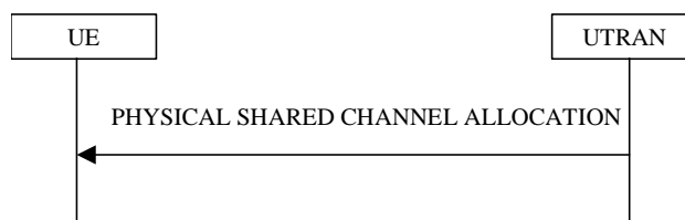
Figure 34: Physical Shared Channel Allocation
