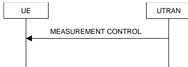
Figure 56: Measurement Control, normal case
