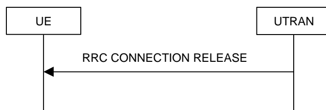
Figure 8.1.4-2: RRC Connection Release procedure on the CCCH
