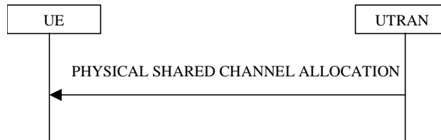
Figure 8.2.7-1: Physical Shared Channel Allocation
