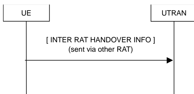
Figure 8.1.16-1: Inter RAT handover information transfer, normal flow
