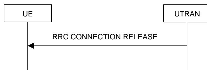
Figure 8.1.4-2: RRC Connection Release procedure on the CCCH
