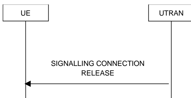
Figure 8.1.13-1: Signalling connection release procedure, normal case
