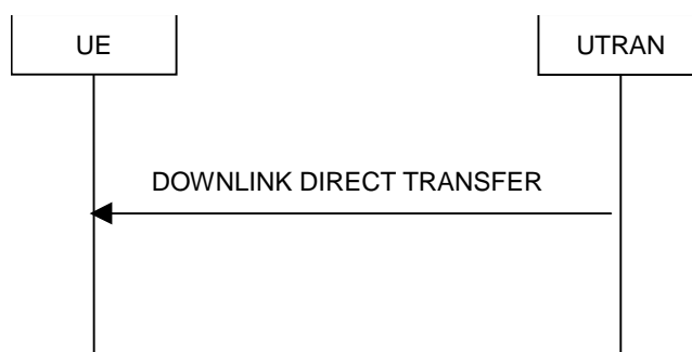
Figure 8.1.9-1: Downlink Direct transfer, normal flow
