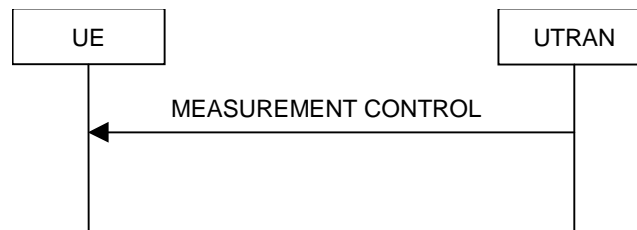
Figure 8.4.1-1: Measurement Control, normal case
