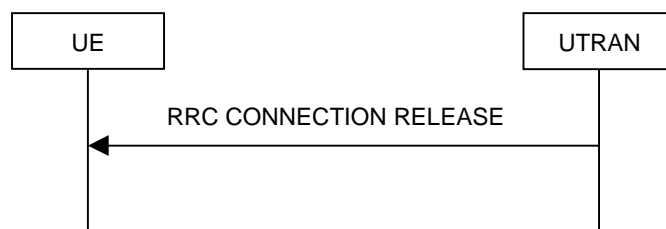
Figure 8.1.4-2: RRC Connection Release procedure on the CCCH
