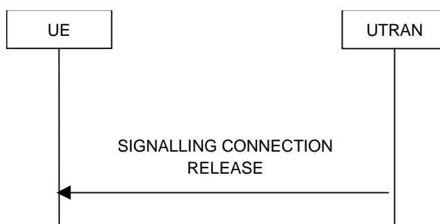
Figure 8.1.13-1: Signalling connection release procedure, normal case
