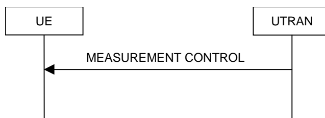
Figure 8.4.1-1: Measurement Control, normal case
