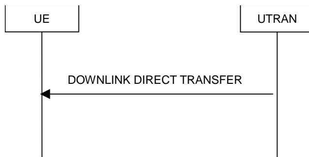
Figure 8.1.9-1: Downlink Direct transfer, normal flow
