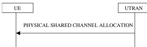
Figure 8.2.7-1: Physical Shared Channel Allocation
