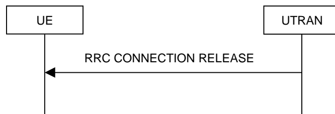
Figure 8.1.4-2: RRC Connection Release procedure on the CCCH
