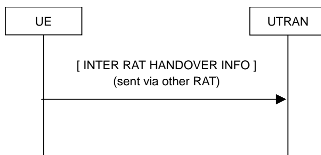
Figure 8.1.16-1: Inter RAT handover information transfer, normal flow
