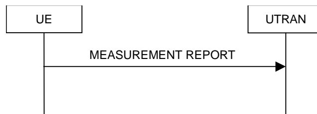
Figure 8.4.2-1: Measurement report, normal case
