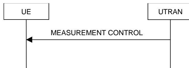
Figure 8.4.1-1: Measurement Control, normal case
