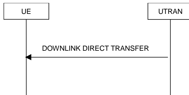
Figure 8.1.9-1: Downlink Direct transfer, normal flow
