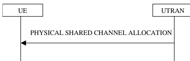
Figure 8.2.7-1: Physical Shared Channel Allocation
