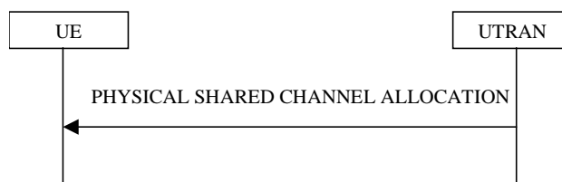
Figure 8.2.7-1: Physical Shared Channel Allocation
