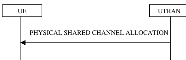
Figure 8.2.7-1: Physical Shared Channel Allocation
