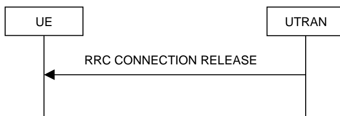
Figure 8.1.4-2: RRC Connection Release procedure on the CCCH
