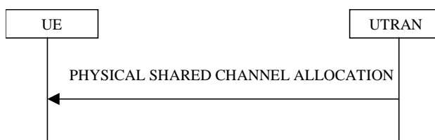
Figure 8.2.7-1: Physical Shared Channel Allocation
