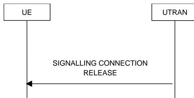
Figure 8.1.13-1: Signalling connection release procedure, normal case
