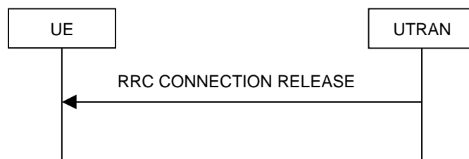
Figure 8.1.4-2: RRC Connection Release procedure on the CCCH
