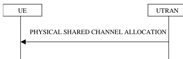
Figure 8.2.7-1: Physical Shared Channel Allocation
