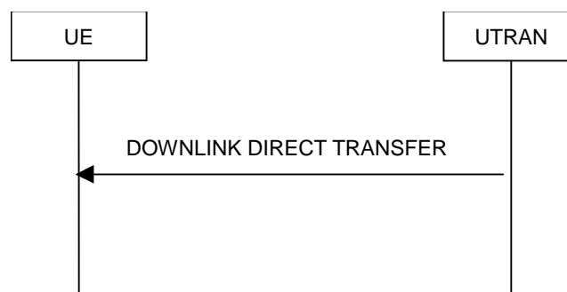
Figure 8.1.9-1: Downlink Direct transfer, normal flow
