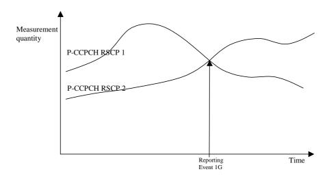
Figure 14.1.3.1-1: A P-CCPCH RSCP becomes better than the previous best P-CCPCH RSCP
