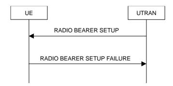
Figure 8.2.2-2: Radio Bearer Establishment, failure case
