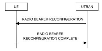
Figure 8.2.2-3: Radio bearer reconfiguration, normal flow
