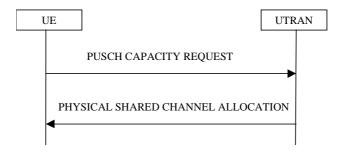
Figure 8.2.8-1: PUSCH Capacity request procedure
