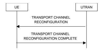
Figure 8.2.2-7: Transport channel reconfiguration, normal flow
