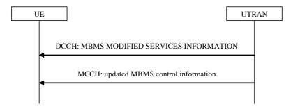
Figure 8.7.3-2: MBMS notification on DCCH
