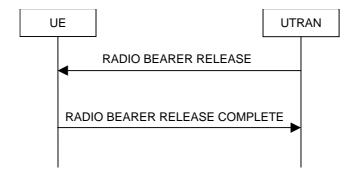
Figure 8.2.2-5: Radio Bearer Release, normal case
