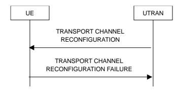
Figure 8.2.2-8: Transport channel reconfiguration, failure case
