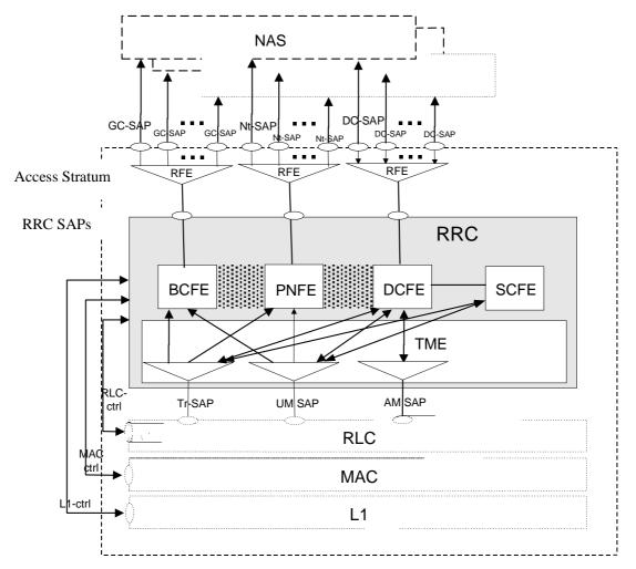
Figure 4.2-1: UE side model of RRC
