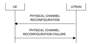
Figure 8.2.2-10: Physical channel reconfiguration, failure case
