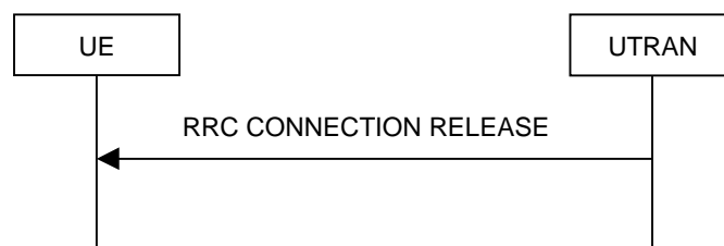
Figure 8.1.4-2: RRC Connection Release procedure on the CCCH
