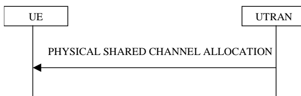
Figure 8.2.7-1: Physical Shared Channel Allocation
