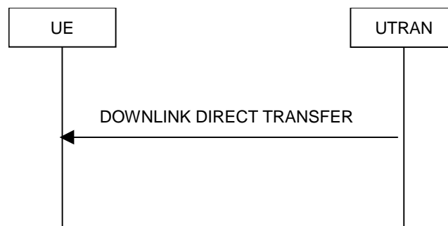
Figure 8.1.9-1: Downlink Direct transfer, normal flow
