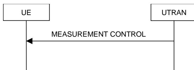
Figure 8.4.1-1: Measurement Control, normal case
