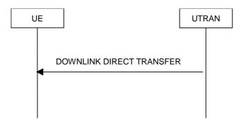
Figure 8.1.9-1: Downlink Direct transfer, normal flow
