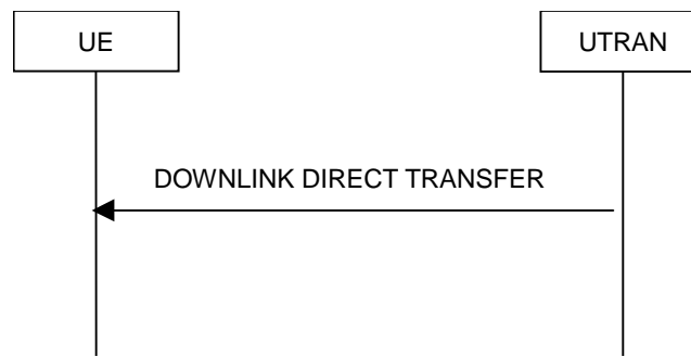
Figure 8.1.9-1: Downlink Direct transfer, normal flow
