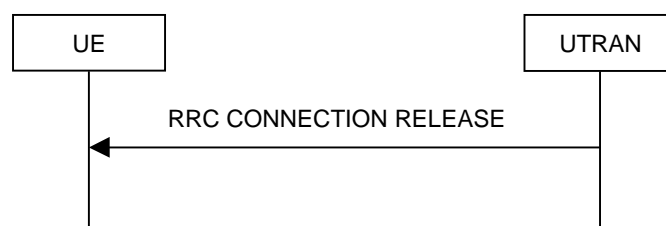
Figure 8.1.4-2: RRC Connection Release procedure on the CCCH
