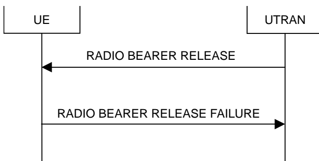
Figure 8.2.2-6: Radio Bearer Release, failure case
