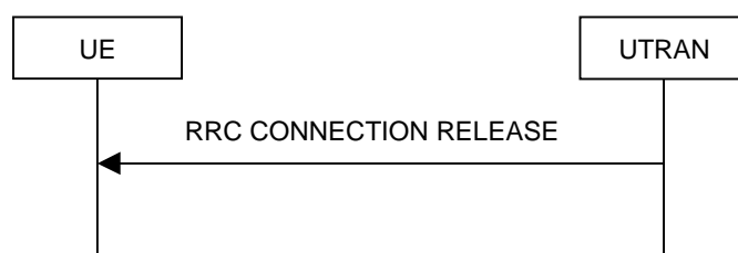
Figure 8.1.4-2: RRC Connection Release procedure on the CCCH
