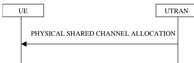
Figure 8.2.7-1: Physical Shared Channel Allocation
