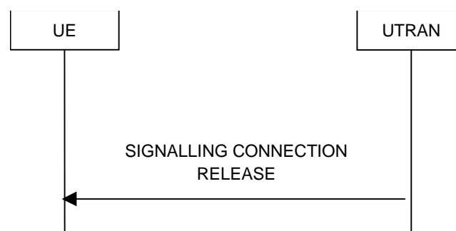
Figure 8.1.13-1: Signalling connection release procedure, normal case
