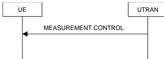
Figure 8.4.1-1: Measurement Control, normal case
