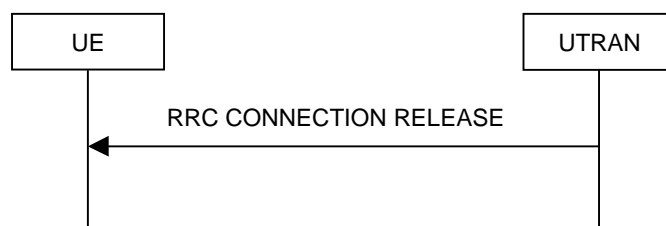
Figure 8.1.4-2: RRC Connection Release procedure on the CCCH
