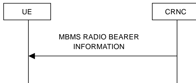
Figure 8.3.3: MBMS radio bearer information signalling flow
