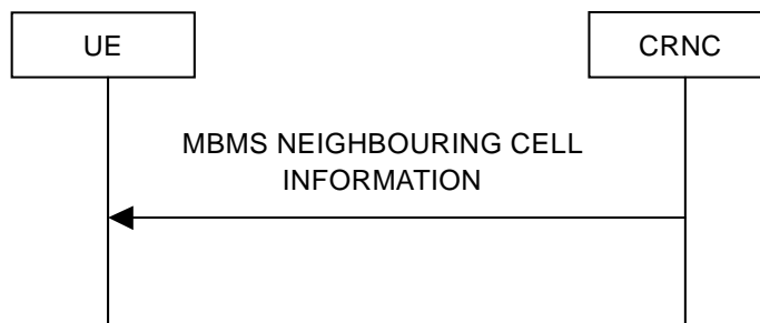
Figure 8.3.5: MBMS Neighbouring Cell Information signalling flow
