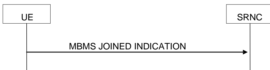
Figure 8.3.6: MBMS joined indication signalling flow
