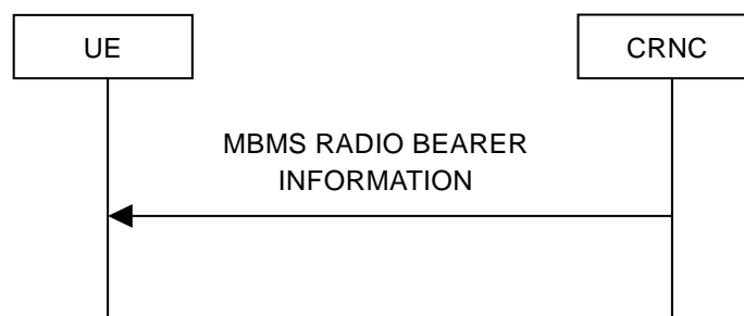
Figure 8.3.3: MBMS radio bearer information signalling flow
