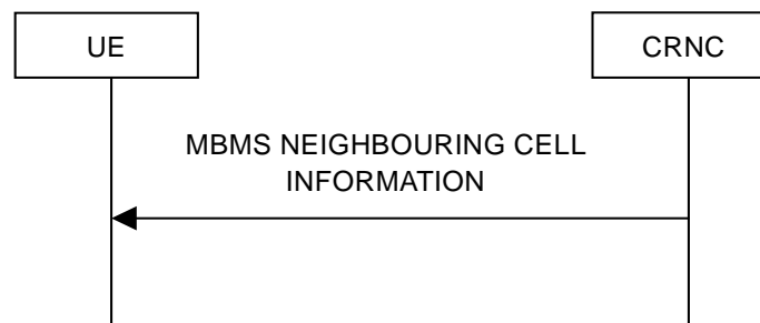
Figure 8.3.5: MBMS Neighbouring Cell Information signalling flow
