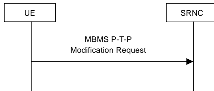
Figure 8.3.9: MBMS P-T-P Modification Request.
