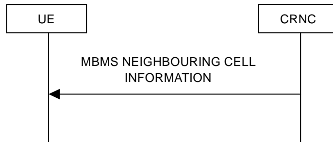
Figure 35: MBMS Neighbouring Cell Information signalling flow
