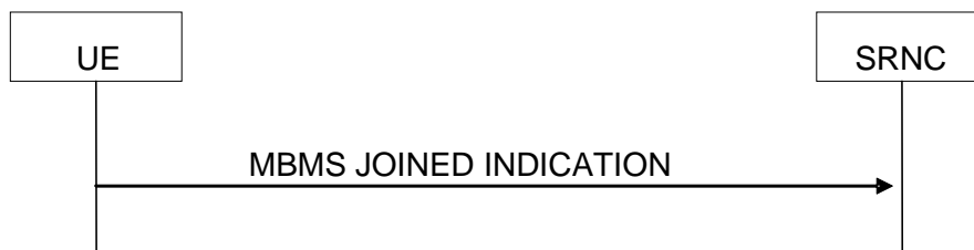
Figure 36: MBMS joined indication signalling flow
