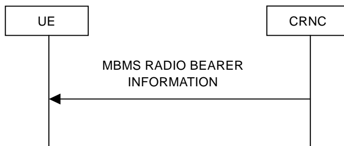
Figure 8.3.3: MBMS radio bearer information signalling flow
