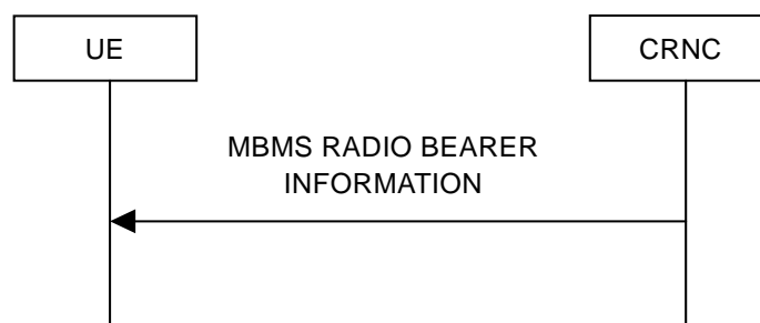
Figure 8.3.3: MBMS radio bearer information signalling flow
