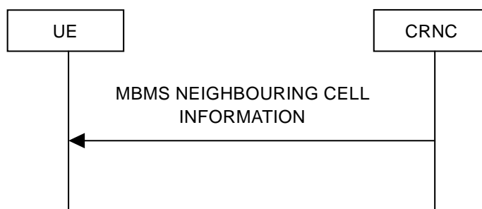
Figure 8.3.5: MBMS Neighbouring Cell Information signalling flow
