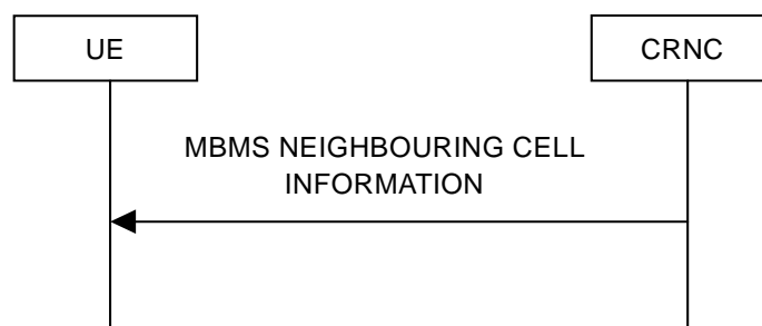
Figure 8.3.5: MBMS Neighbouring Cell Information signalling flow
