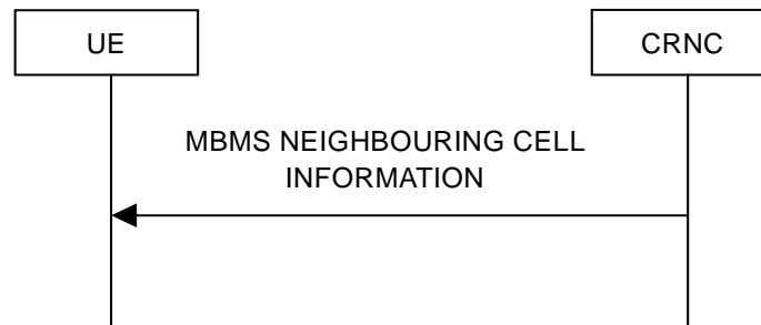
Figure 8.3.5: MBMS Neighbouring Cell Information signalling flow
