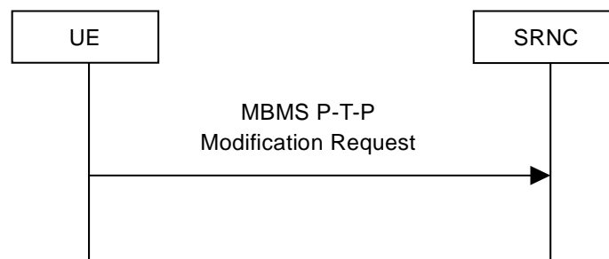
Figure 8.3.9: MBMS P-T-P Modification Request.
