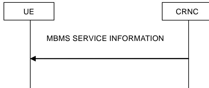
Figure 8.3.2: MBMS service information signalling flow
