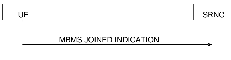
Figure 8.3.6: MBMS joined indication signalling flow
