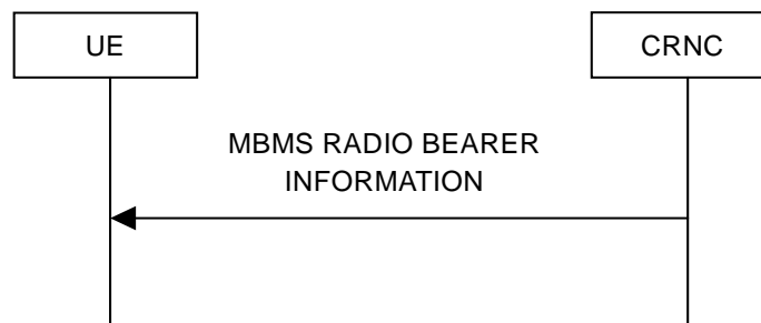
Figure 8.3.3: MBMS radio bearer information signalling flow
