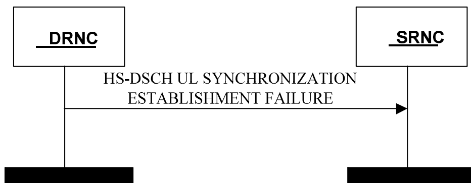
Figure 4AC: HS-DSCH UL Synchronization Establishment Failure procedure
