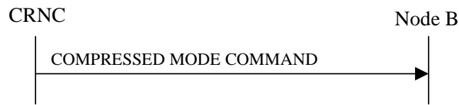
Figure 47: Compressed Mode Command procedure, Successful Operation
