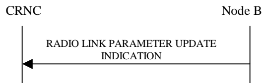
Figure 48: Radio Link Parameter Update Indication, Successful Operation
