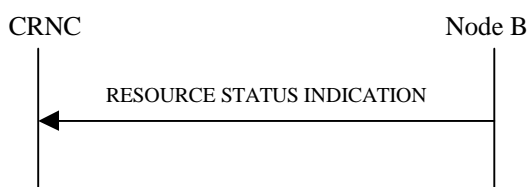
Figure 21: Resource Status Indication procedure, Successful Operation
