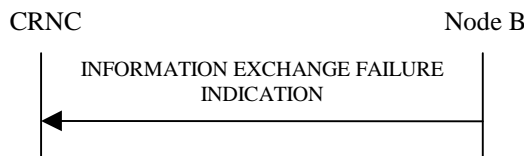
Figure 27P: Information Exchange Failure procedure, Successful Operation
