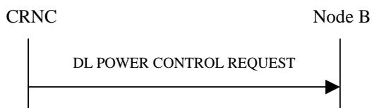
Figure 37: Downlink Power Control procedure, Successful Operation
