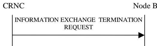
Figure 27O: Information Exchange Termination procedure, Successful Operation
