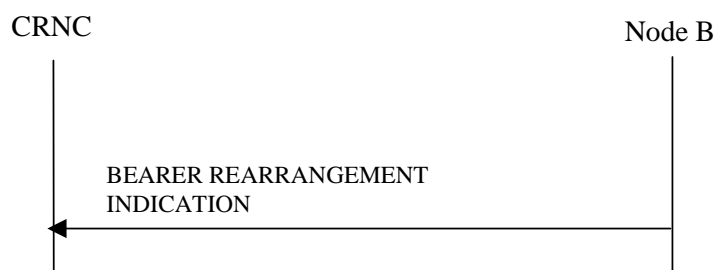
Figure 47C: Bearer Re-arrangement Indication, Successful Operation
