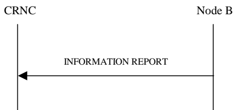
Figure 27N: Information Reporting procedure, Successful Operation
