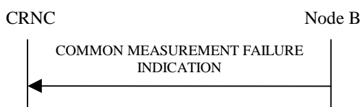
Figure 15: Common Measurement Failure procedure, Successful Operation
