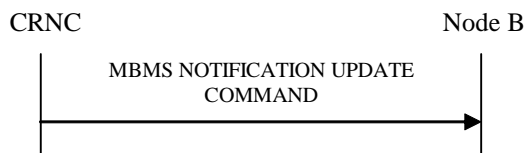
Figure 27Q: MBMS Notification Update procedure, Successful Operation
