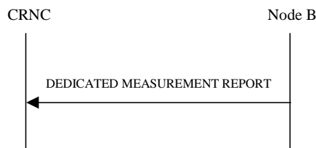
Figure 40: Dedicated Measurement Reporting procedure, Successful Operation
