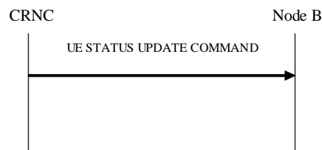
Figure 27R: UE Status Update procedure, Successful Operation
