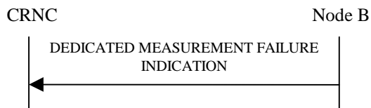
Figure 42: Dedicated Measurement Failure procedure, Successful Operation
