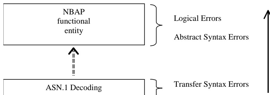
Figure 38: Protocol Errors in NBAP.
