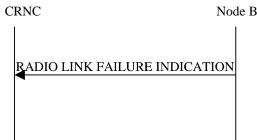
Figure 43: Radio Link Failure procedure, Successful Operation
