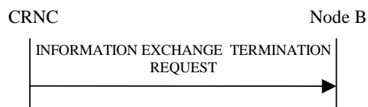
Figure 27O: Information Exchange Termination procedure, Successful Operation
