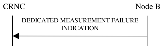
Figure 42: Dedicated Measurement Failure procedure, Successful Operation
