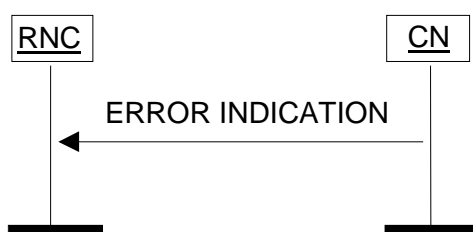
Figure 31: Error Indication procedure, CN originated. Successful operation.
