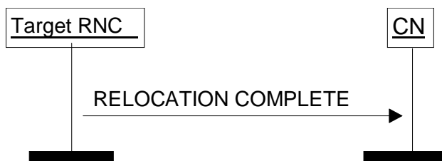
Figure 10: Relocation Complete procedure. Successful operation.
