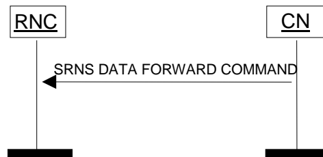
Figure 13: SRNS Data Forwarding Initiation procedure. Successful operation.
