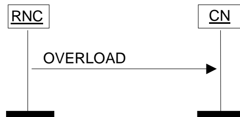
Figure 28: Overload at the UTRAN. Successful operation.
