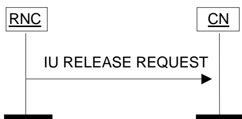
Figure 3: Iu Release Request procedure. Successful operation.
