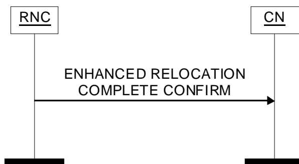
Figure 70: Enhanced Relocation Complete Confirm procedure. Successful operation.
