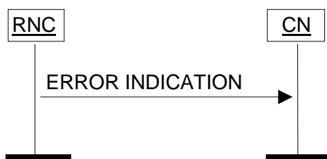
Figure 32: Error Indication procedure, RNC originated. Successful operation.
