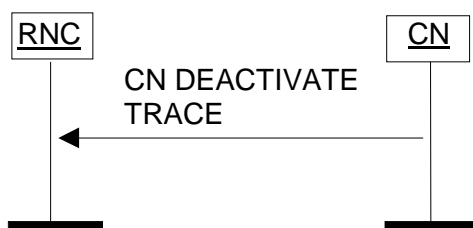
Figure 33: CN Deactivate Trace procedure. Successful operation.
