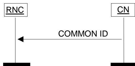
Figure 17: Common ID procedure. Successful operation.
