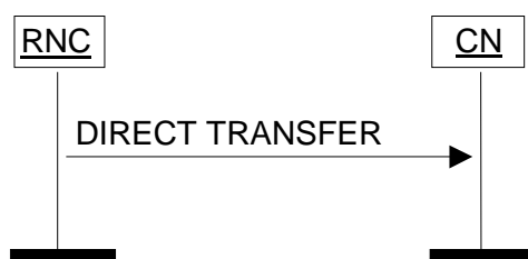
Figure 26: Direct Transfer, RNC originated. Successful operation.
