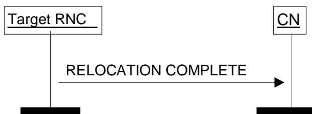
Figure 10: Relocation Complete procedure. Successful operation.
