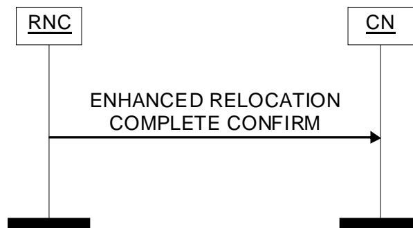
Figure 70: Enhanced Relocation Complete Confirm procedure. Successful operation.
