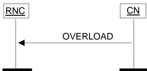
Figure 27: Overload at the CN. Successful operation.
