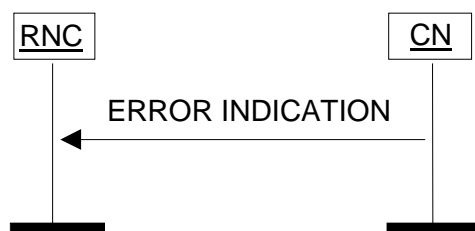
Figure 31: Error Indication procedure, CN originated. Successful operation.
