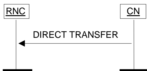
Figure 25: Direct Transfer, CN originated. Successful operation.
