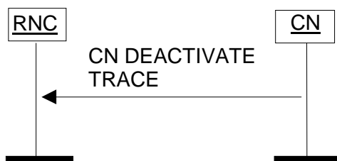
Figure 33: CN Deactivate Trace procedure. Successful operation.
