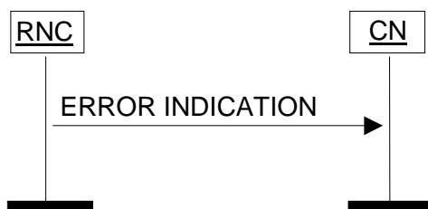
Figure 32: Error Indication procedure, RNC originated. Successful operation.
