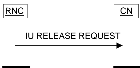
Figure 3: Iu Release Request procedure. Successful operation.
