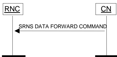
Figure 13: SRNS Data Forwarding Initiation procedure. Successful operation.
