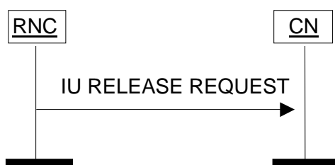
Figure 3: Iu Release Request procedure. Successful operation.
