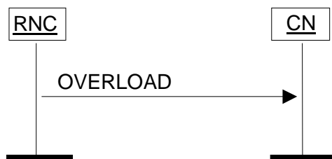
Figure 28: Overload at the UTRAN. Successful operation.
