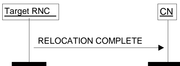
Figure 10: Relocation Complete procedure. Successful operation.
