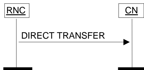
Figure 26: Direct Transfer, RNC originated. Successful operation.
