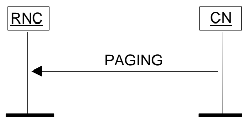
Figure 16: Paging procedure. Successful operation.
