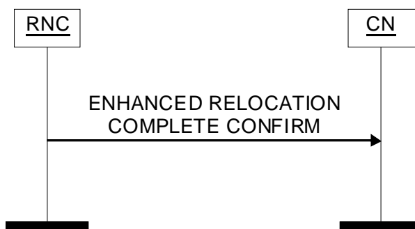
Figure 70: Enhanced Relocation Complete Confirm procedure. Successful operation.
