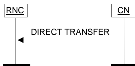
Figure 25: Direct Transfer, CN originated. Successful operation.
