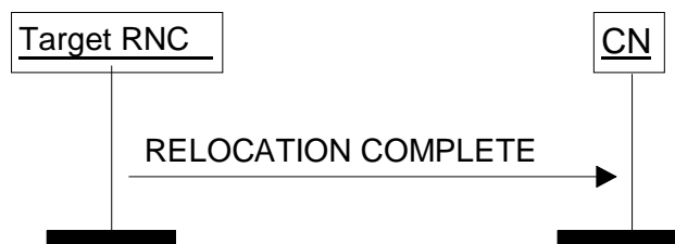
Figure 10: Relocation Complete procedure. Successful operation.
