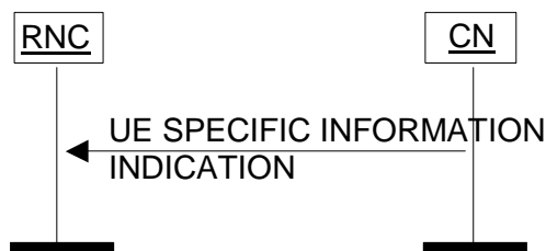
Figure 41: UE Specific Information procedure. Successful operation.
