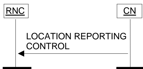
Figure 21: Location Reporting Control procedure. Successful operation.
