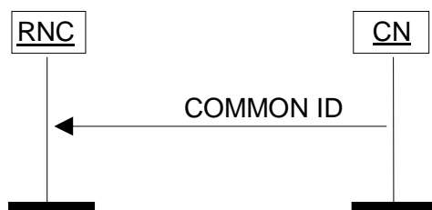
Figure 17: Common ID procedure. Successful operation.
