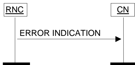
Figure 32: Error Indication procedure, RNC originated. Successful operation.
