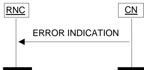
Figure 31: Error Indication procedure, CN originated. Successful operation.
