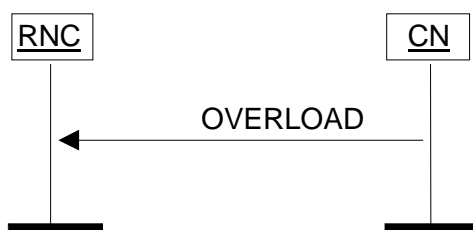
Figure 27: Overload at the CN. Successful operation.
