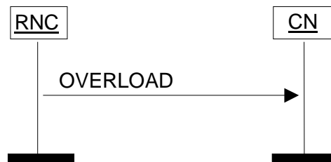
Figure 28: Overload at the UTRAN. Successful operation.
