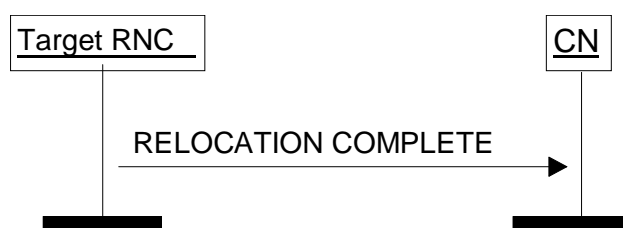
Figure 10: Relocation Complete procedure. Successful operation.
