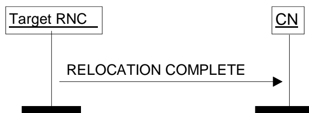
Figure 10: Relocation Complete procedure. Successful operation.
